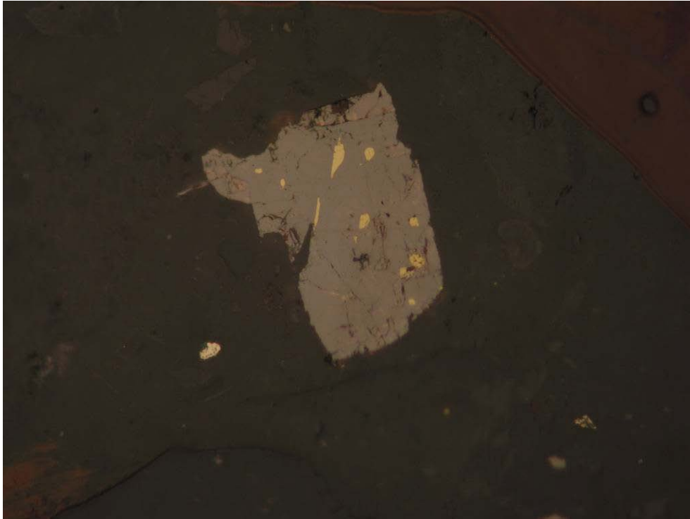
Figure B17: Photomicrograph of a liberated grain of sphalerite with inclusions of chalcopyrite in sample 11. RL, FOV = ~ 0.28 mm.
