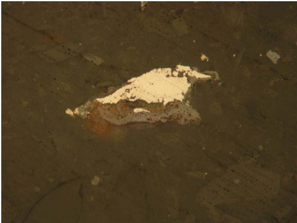
Figure 6: Photomicrograph of a liberated grain of pyrite, partially rimmed by hematite. RL, FOV = ~ 0.27 mm.
