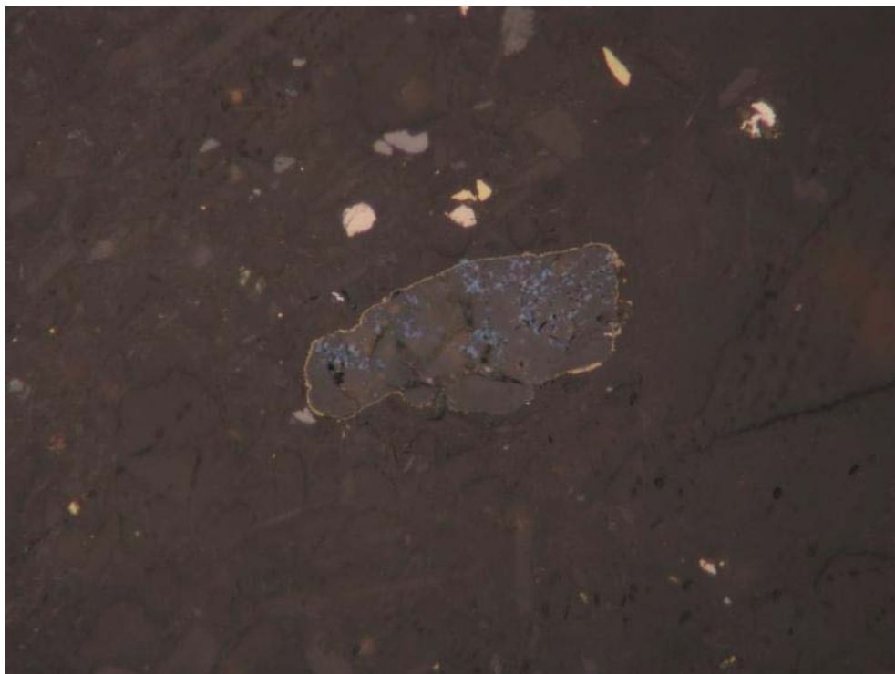
Figure 4: Close-up of sample 3 showing the occurrence of chalcopyrite and covellite. In photomicrograph A, a liberated chalcopyrite grain is rimmed by covellite. In B, a gangue mineral is pitted by covellite and rimmed by chalcopyrite. RL, FOV= ~ 0.28 mm.
